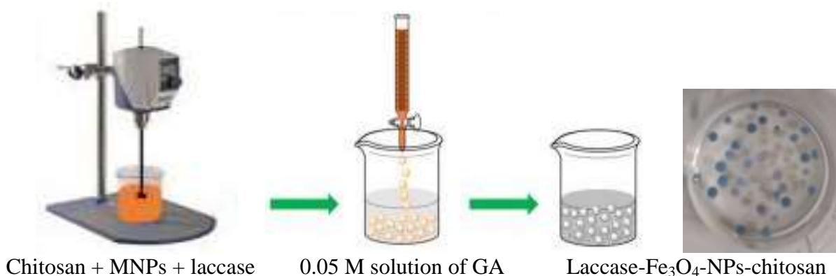
Fig. 8. Schematic diagram of the formation of chitosan beads with encapsulated bioelement: laccase-Fe 3 O 4 -NPs
