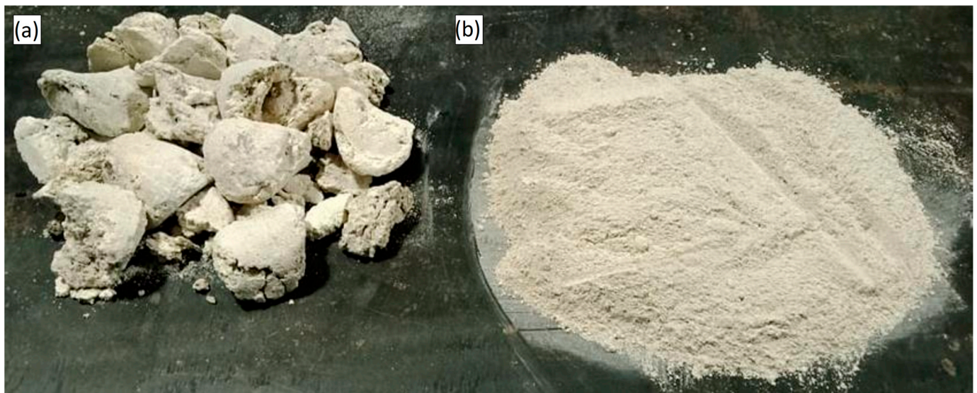
Figure 1. The appearance of WSA: (a) primary form; (b) crushed into a filler aggregate.
