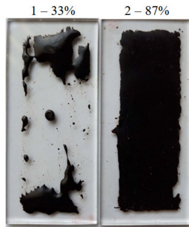
Figure 5. The glass plates after testing two bitumen samples for adhesion to the glass surface, 33 and 87%, respectively.
