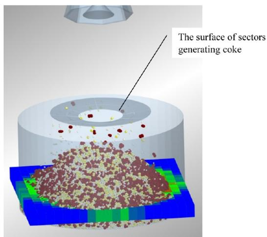
Figure 21. Creation of the backfill surface.
