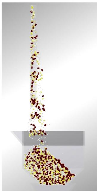
**Figure 2.** Coke-directed bucket imitation model, which is located above the coke-carrying railcar during coke discharge.
