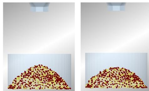
Immediately after filling in the tray After shrinkage in 7 seconds
