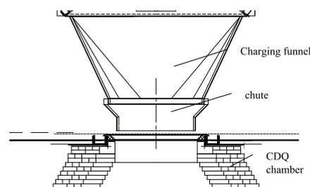
**Figure 4.** Real coke charging device of PrJSC “Avdiivka Coke”.
