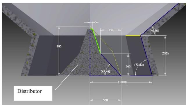
Figure 16. Changed coke distributor and funnel hole.
