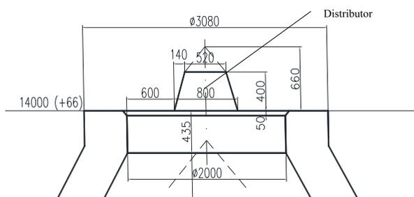
Figure 11. First design of the coke distributor in the funnel of the loading hole.
