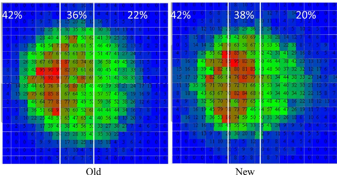
Figure 15. Comparison of particle distribution at the end of the experiment with old and new charging devices. Class of small (-60 mm) particles.
