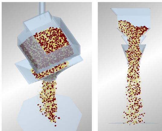
Figure 6. Start of coke charging into the CDQ chamber.
