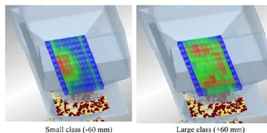
Figure 17. Coke size distribution during discharge from the railcar (number of particles indicated by color: red—79÷95, brown—68÷78, light green—43÷67, dark green—27÷42, dark blue—5÷10).
