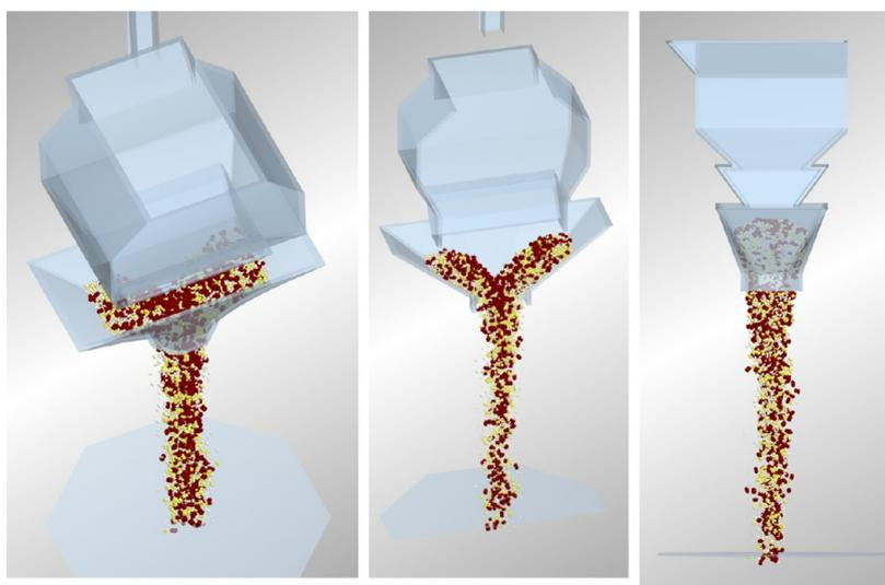
Figure 7. End of coke charging.
