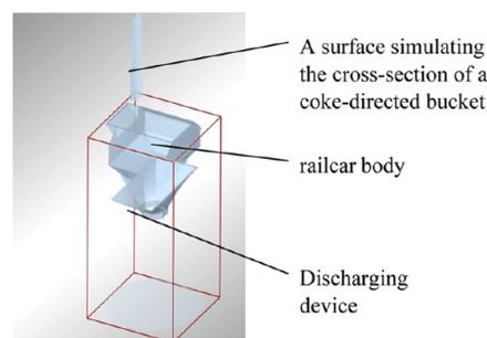
Figure 1. Installation model.
