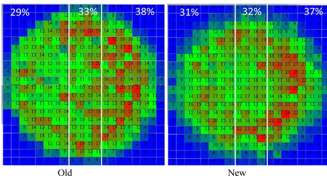
Figure 14. Comparison of particle distribution at the end of the experiment with old and new charging devices. Class of large (+60 mm) particles.
