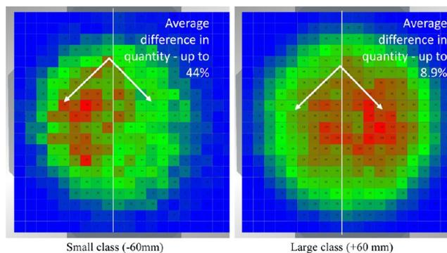
Figure 9. Distribution of coke pieces immediately after filling in the tray on the embankment lower part.
