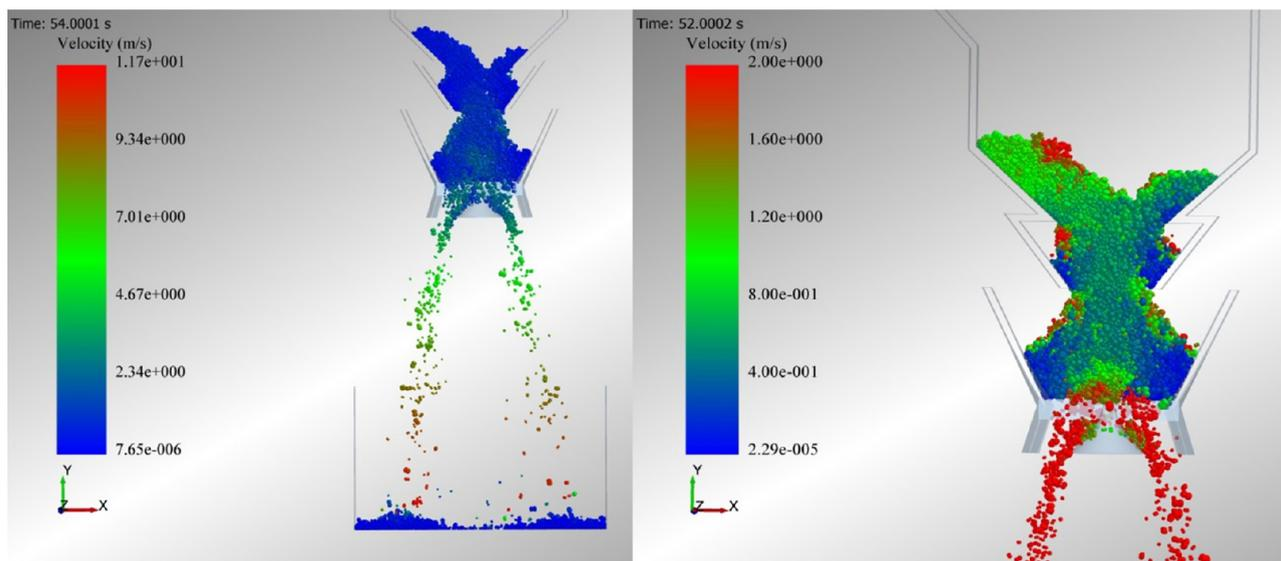
Figure 20. Fall velocity of particles.
