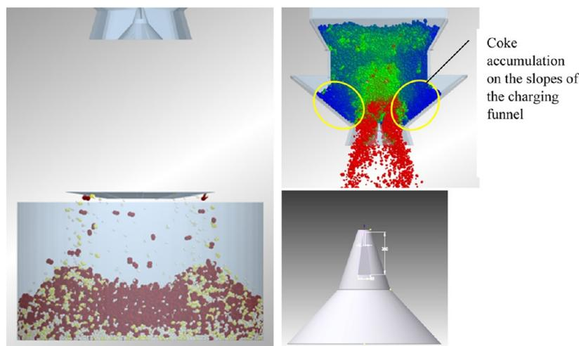
**Figure 25.** Formation of the saddle-shaped gap.
