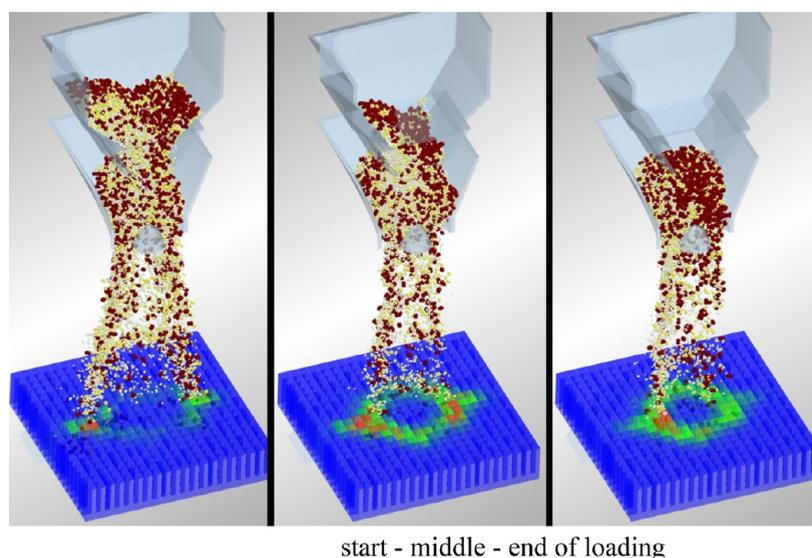
Figure 12. Stages of coke descent through the proposed distributor.
