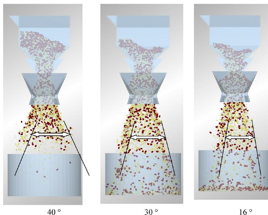
**Figure 19.** Change in particle dispersion angle during coke discharging.
