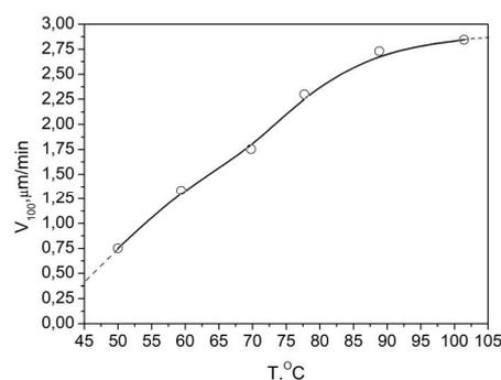
Fig.1. Dependence of the etching rate of silicon in the (100) plane on the temperature in an aqueous KOH solution.
