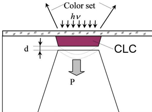
Fig.3. Schematic representation of a microelectronic label-sensor for optical identification: CLC- cholesteric liquid crystal, P-pressure, d- membrane thickness.
